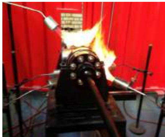
Test valve during burn period
